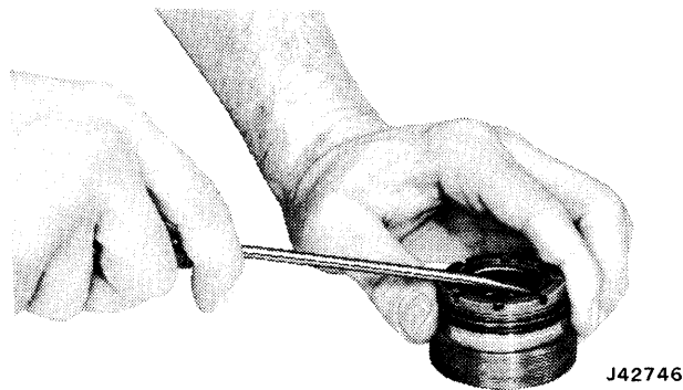
Fig. 11-74 Removing Thrust Bearing Retainer
