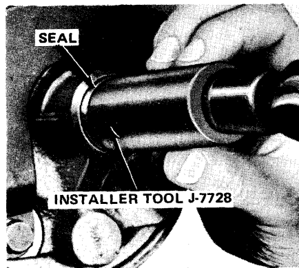
Fig. 11-98 Installing Pump Shaft Seal
