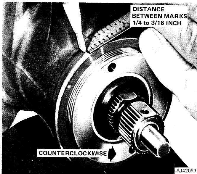
Fig. 11-93 Remarking Housing
