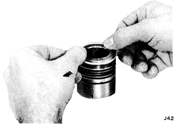
Fig. 11-86 Installing Valve Body Seal Rings
