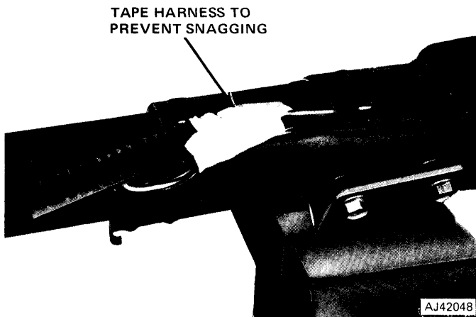
Fig. 11-25 Removing Turn Signal Switch Harness
